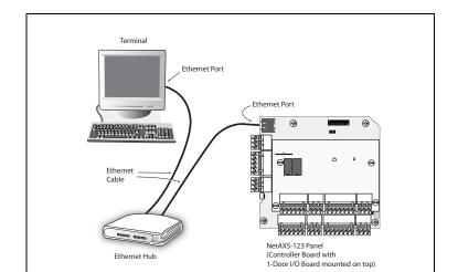
Figure 1-1: NetAXS-123 Web Server Hub Connection
